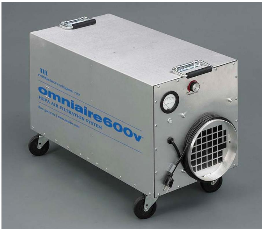
The **OMNIAIRE 600V** HEPA Air Filtration system is a variable speed HEPA-filtered negative air machine designed for removal of toxic mold, asbestos or other airborne contaminants during construction, renovation and abatement projects or for use with the Mintie Technologies Environmental Containment Unit (ECU) to create HEPA-filtered negative pressure environments.
