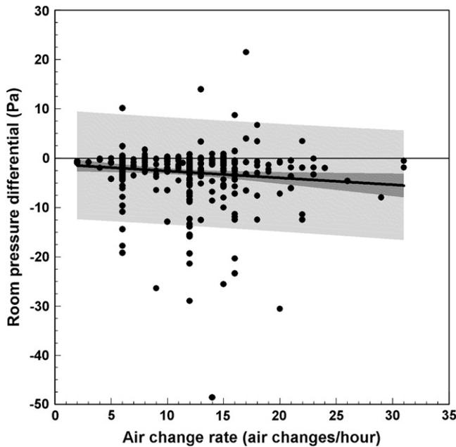
**Fig 1.** Pressure differential versus air changes per hour. The thick line represents the regression between the 2 variables. The dark shaded region is the 95% confidence band for the mean value of pressure differential at each air-change rate. The light shaded region is the 95% prediction band for an individual room's pressure differential if the air-change rate for the room is known.
