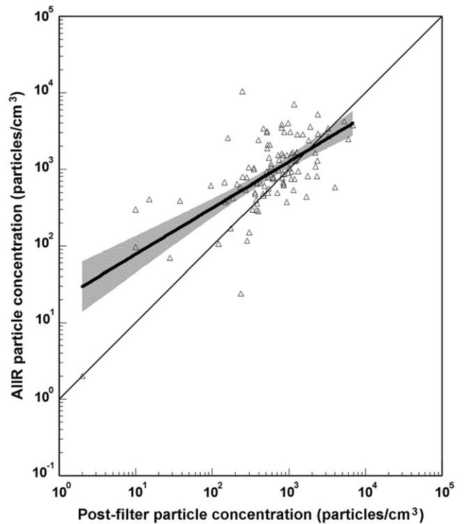
**Fig 2.** Open triangles represent particle concentrations in the AIIRs versus particle concentrations immediately downstream from the filters in the air-handling units serving the AIIRs. The thick line represents the regression between the 2 variables. The shaded region is the 95% confidence band for the regression line. The 1:1 line is also displayed.
