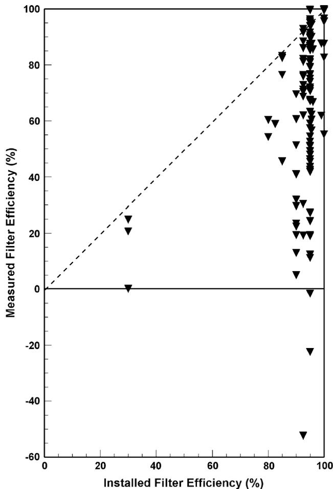
**Fig 4.** Triangles represent measured filter bank efficiency in air-handling units serving AIIRs versus dust spot efficiency reported by manufacturers. The dashed line is a 1:1 relationship between measured efficiency and manufacturer-reported efficiency.
