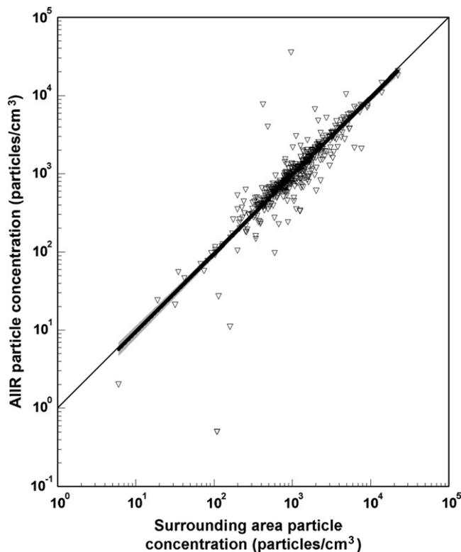
**Fig 3.** Open triangles represent particle concentrations in the AIIRs versus particle concentrations in the areas adjacent to the AIIRs. The thick line represents the regression between the 2 variables. The shaded region is the 95% confidence band for the regression line. The 1:1 line is also displayed.
