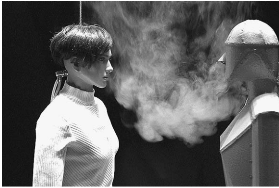
Figure 2 Smoke visualization of exhalation flow from nose of the right mannequin penetrating into the breathing zone of the left mannequin, which are 0.4 m apart. 94 Reproduced from Figure 12 in Reference 94 with the kind permission of Blackwell Publishing.
